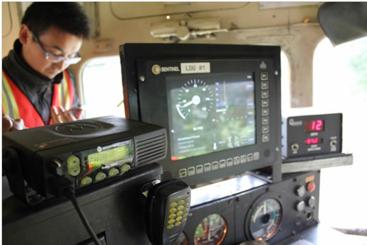
Equipment installed in a Lycoming Valley locomotive is part of a new positive train control system that makers hope will comply with federal requirements. Here the gray band on the speedometer indicates the allowable speed for the track segment. The speedometer will change to yellow as a restriction is approached, then to red when braking is required. The locomotive display unit will then indicate a braking profile to the restricted point.
